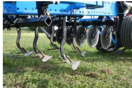
Setting of the Weco-dyn for cover crop destruction and shallow tillage before planting
